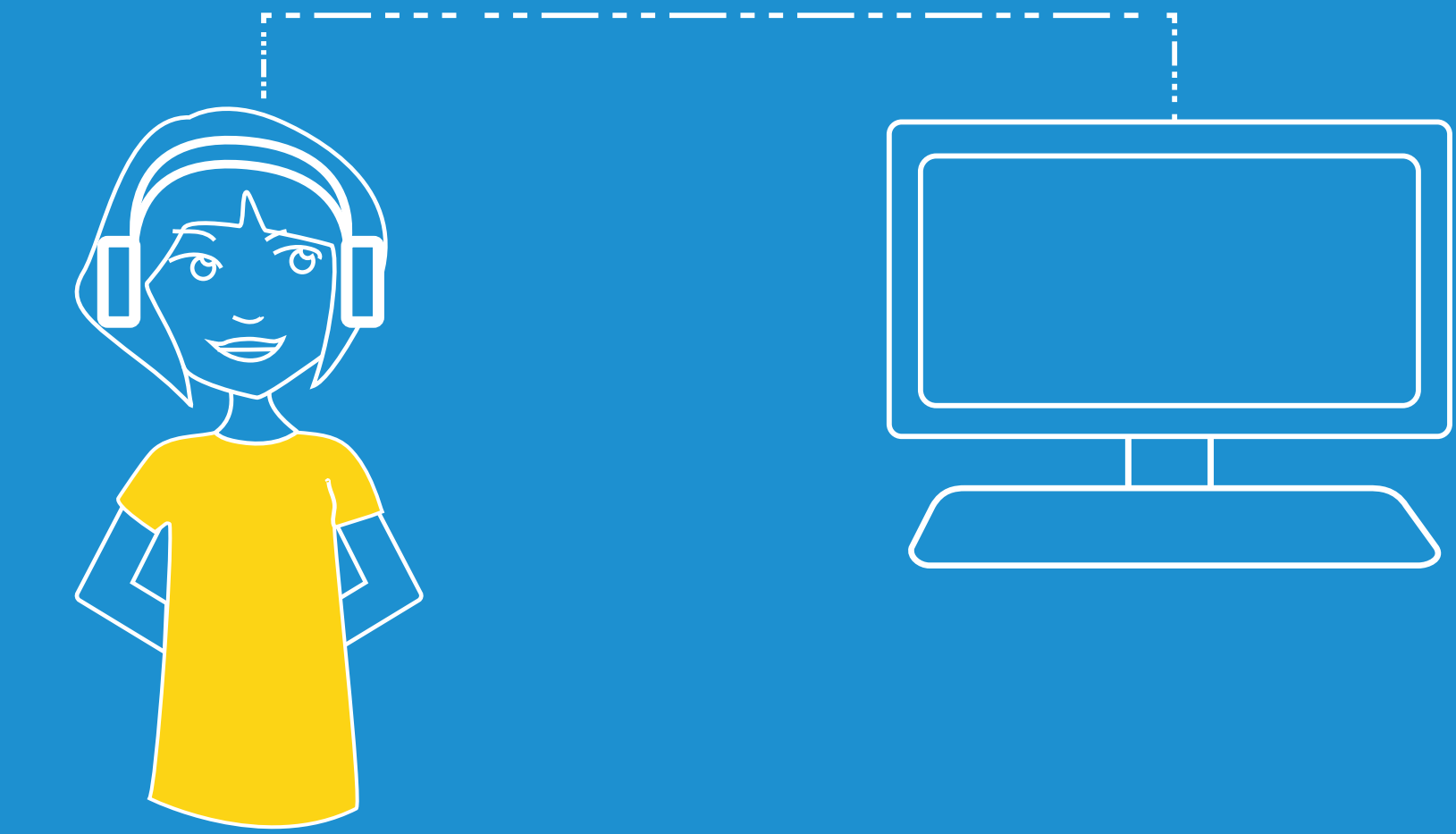
Figure 1: Neurofeedback Training set-up. The portable headset sends EEG data via Bluetooth® to the computer, which performs a Fourier transform and provides feedback directly to the student via game play.
