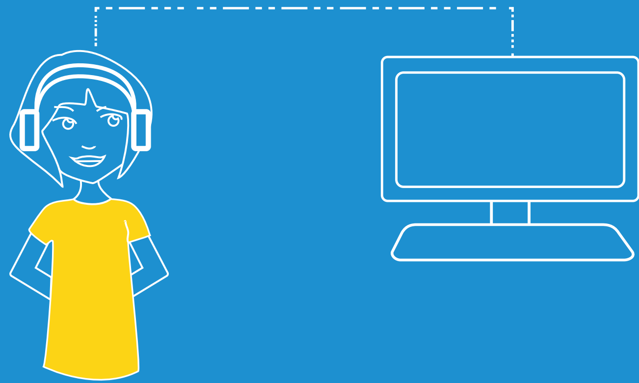
Figure 1: Neurofeedback Training set-up. The portable headset sends EEG data via Bluetooth® to the computer, which performs a Fourier transform and provides feedback directly to the student via game play.
